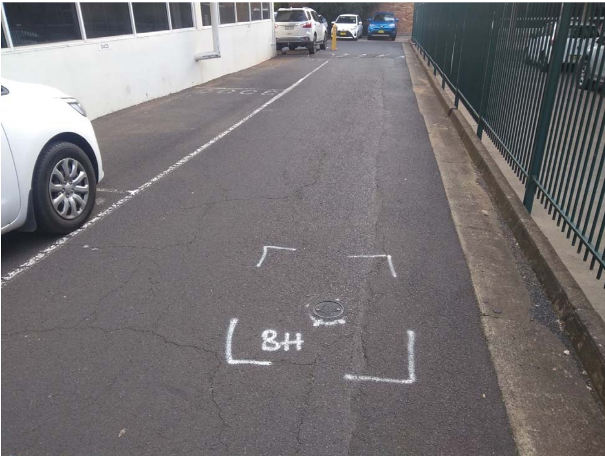
A groundwater monitoring well was identified in the north east corner of 37-39 Carrington Avenue. The monitoring well is believed to have been installed during a recent geotechnical assessment of the site conducted by Macquarie Geotech. The measured static water level in the monitoring well was 13.0m below ground level at the time of the site inspection.
